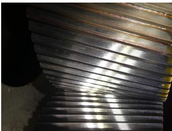
Rad HSS kleine Generatorstufe = i.O
