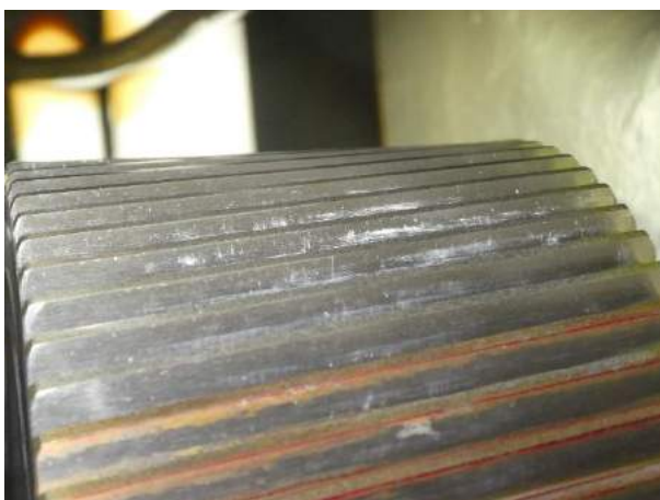
Rad HSS kleine Generatorsstufe = i.O
